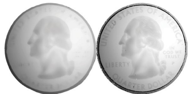
NLOS view of two Quarters, as seen using Gkioulekas' algorithm.
