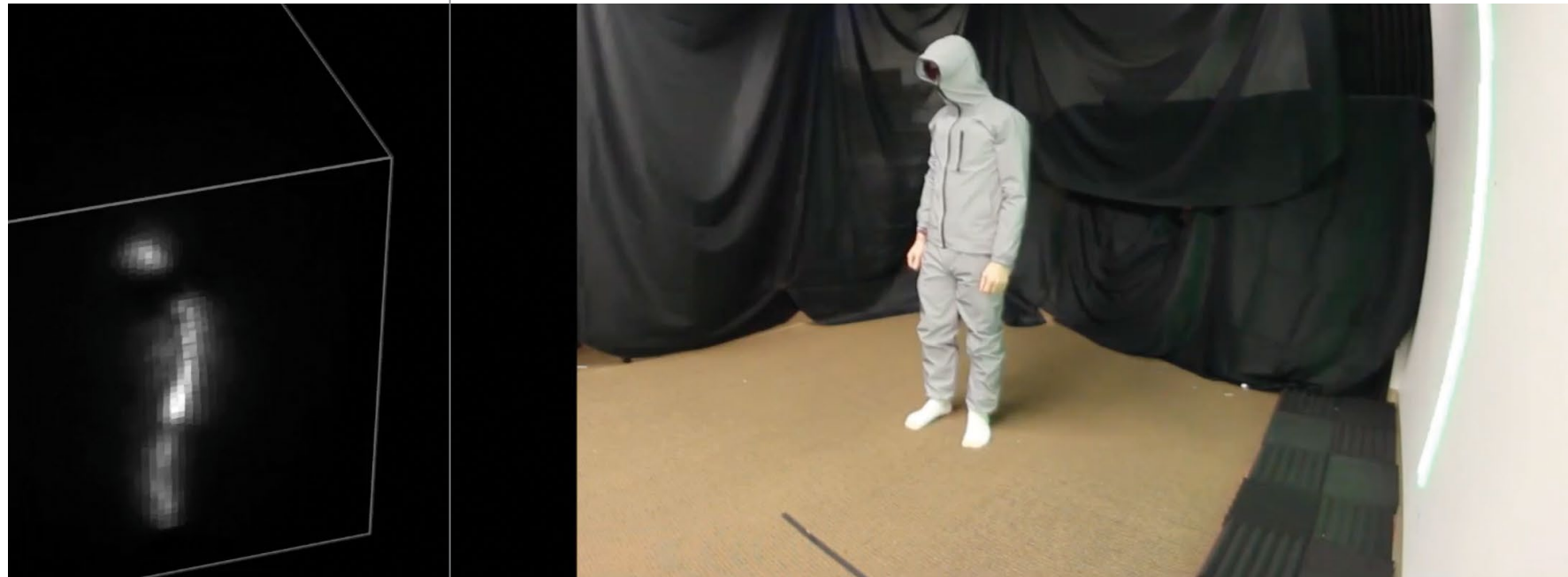
The computer's view (left image) of the person on the right, taken from around a corner as the camera and pulsed laser measure the time photons take to bounce back to the lens.
